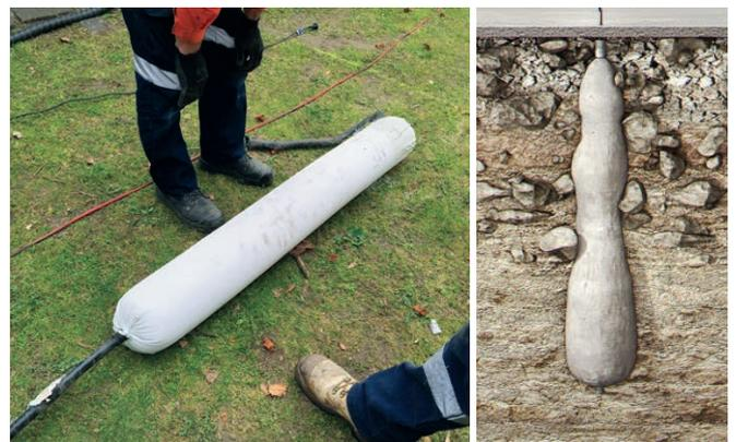
Above: Demonstration of PowerPile free-rise expansion and a diagram of actual installation expansion into ground of varying density.
